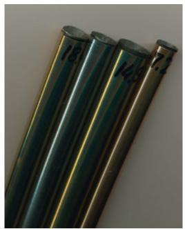
Tubes of braided Carbon Fiber sleeve. Made with hot cured epoxy at 150 degrees C. Glass transition temperature 118 degrees C.
